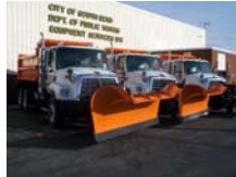
CNG powered Street Dept. Plow Trucks
