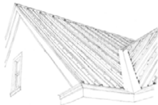
Exposed fastener corrugated metal roofs (top) are not approved in the district. Traditional standing seam (below) may be considered.
