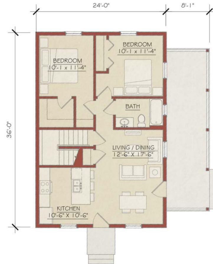
Alternate Ground Floor Plan: Side porch entry option (elevation not shown here) and possible basement stair configuration
