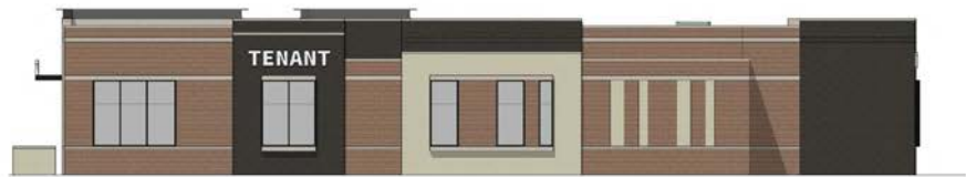
3 EAST ELEVATION Loading/Service Area 1/16" = 1'-0" Total area of calculation zone (Z'-8'): 716sf Total area of vision glass (Z'-8'): 0sf | 0% Total area of nonvision (spandrel) glass (Z'-8'): 104sf Total area of vision and nonvision glass (Z'-8'): 104sf | 15%
