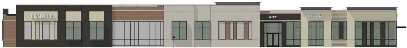
2 NORTH ELEVATION 1/16" = 1'-0" Total area of calculation zone (Z'-8'): 1,166sf Total area of vision glass (Z'-8'): 355sf | 30% Total area of nonvision (spandrel) glass (Z'-8'): 215sf Total area of vision and nonvision glass (Z'-8'): 570sf | 49%
