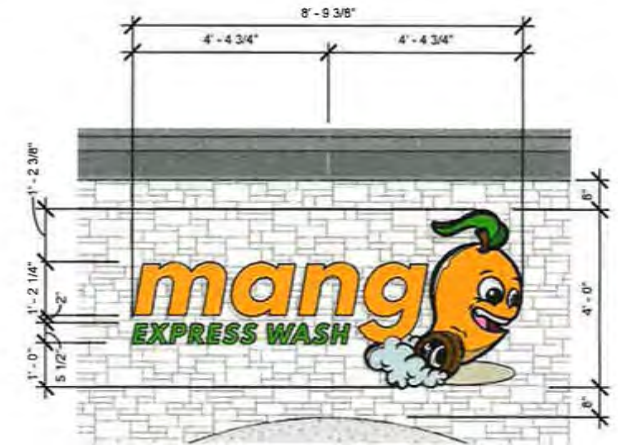
4 BUILDING SIGN (Over Tunnel Doors) SCALE: 3/8" = 1'-0"
