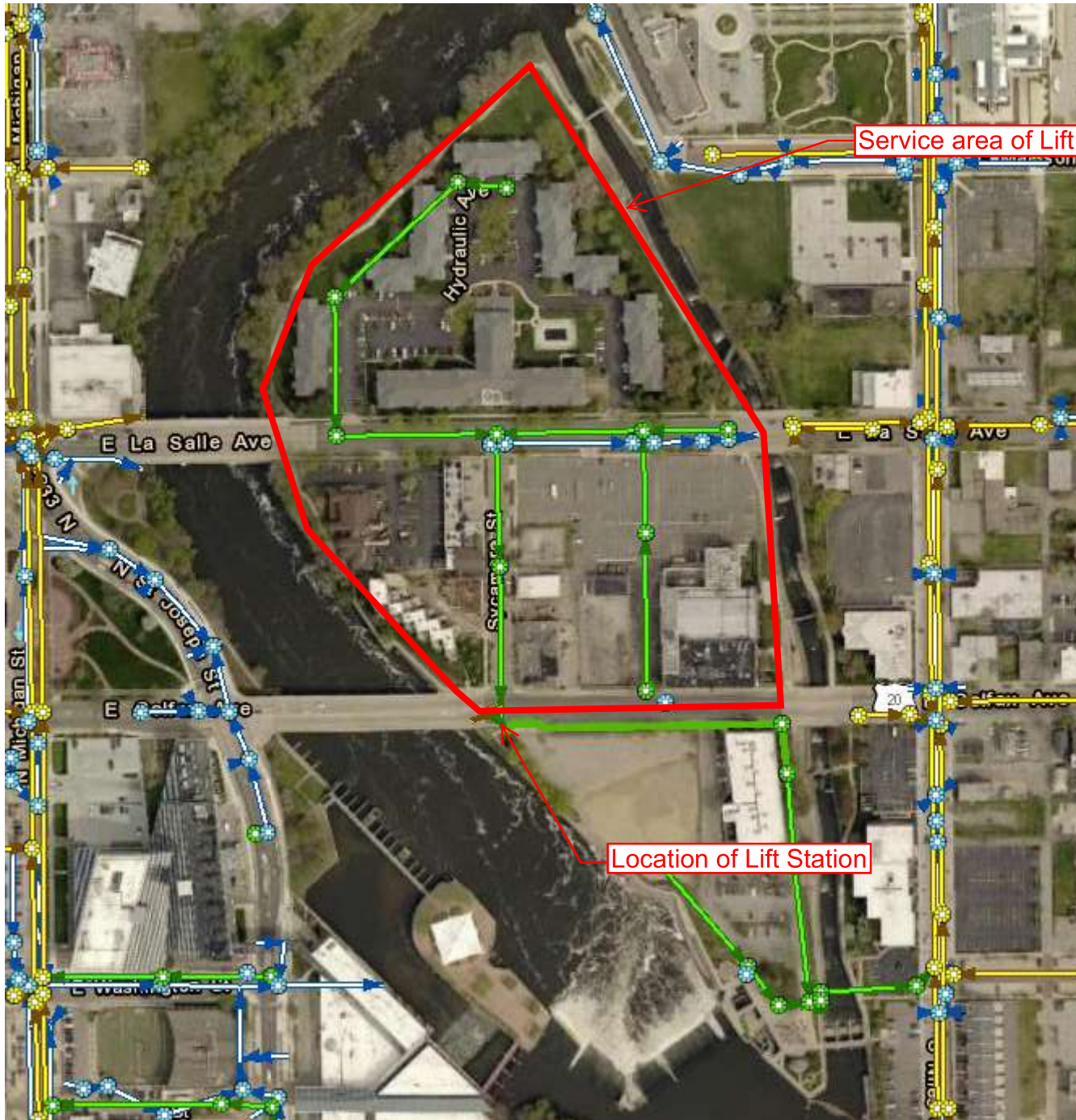
Aerial View of East Race area served by Colfax Lift Station
