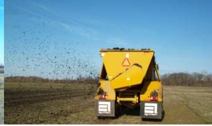
Slinger spreading material on the field
