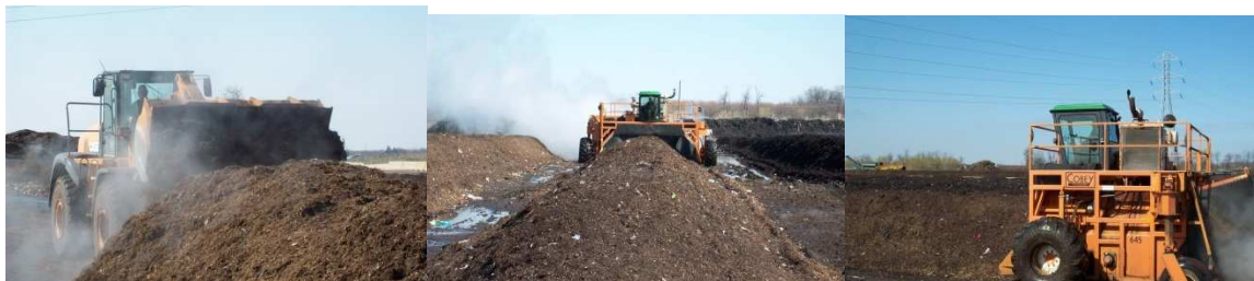
Static piles of compost being turned
