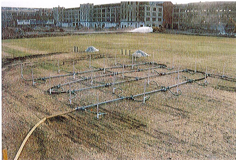
No. 4 – This is an overview of the permanganate injection well field looking to the northeast. The injection well at the far left is IW-A1. The well at the top is IW-E1. The well furthest right is IW-E5. The well at the bottom of the photograph is IW-A5.
