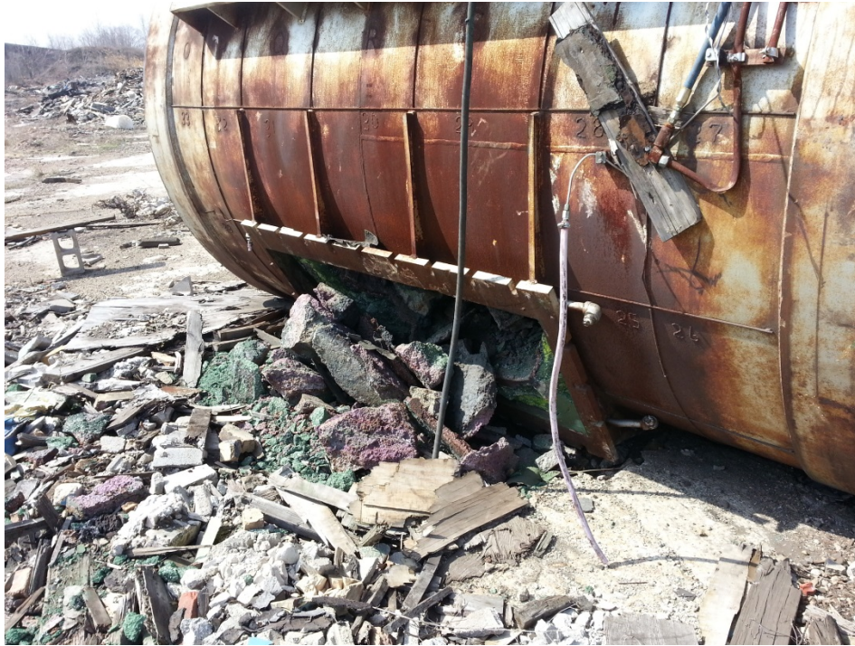
#25: This depicts the backside of the furnace, opposite #22. The multicolored material spilling out is suspected to be chunks of solidified slag or flux.
