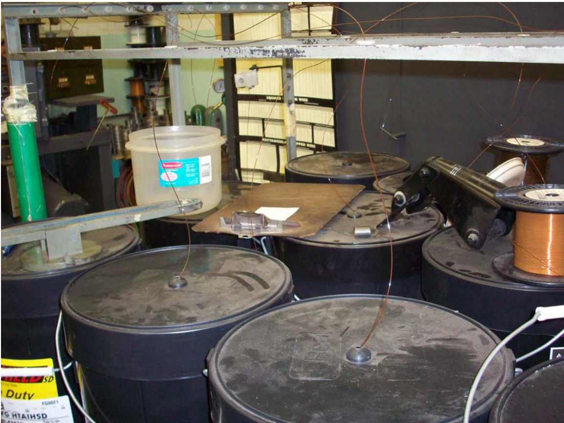
Copper for winding of coils for motors
