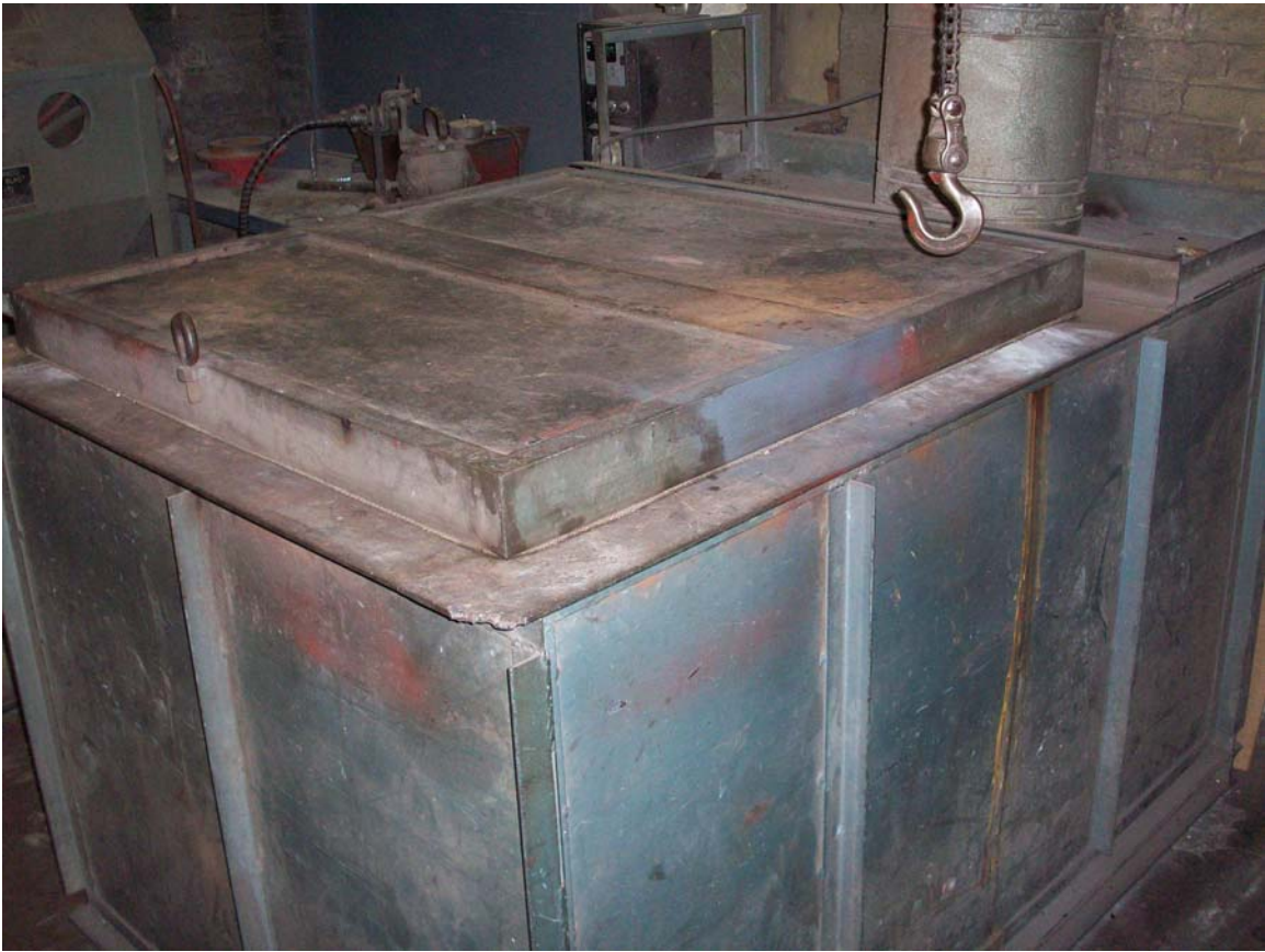
Burn out oven for varnish/enamel removal
