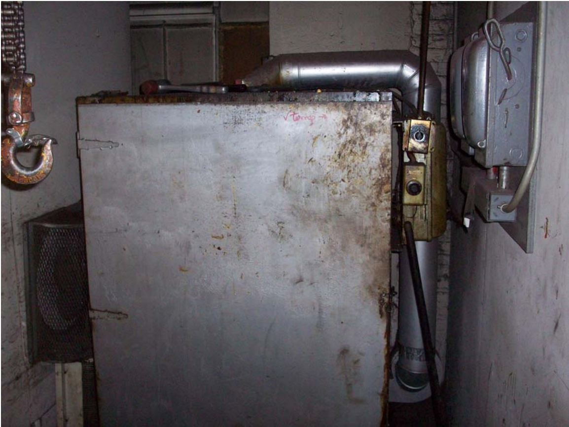
Curing oven for windings ( 325° F for 4-6 hrs)
