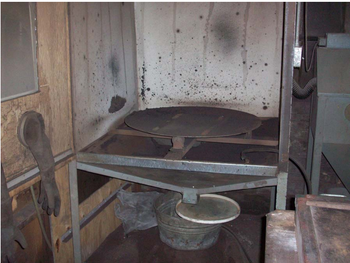
Sandblast area for varnish/enamel removal
