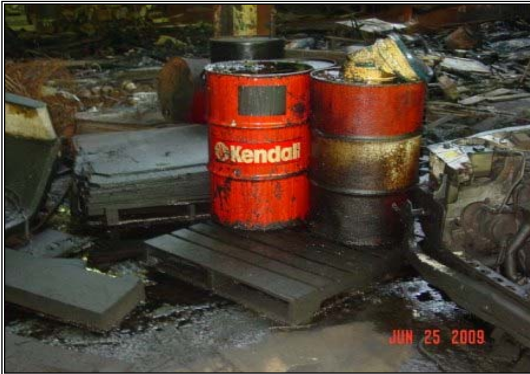
PHOTO 3: Drums in the foundry area that are surrounded by cars and debris have leaked.
