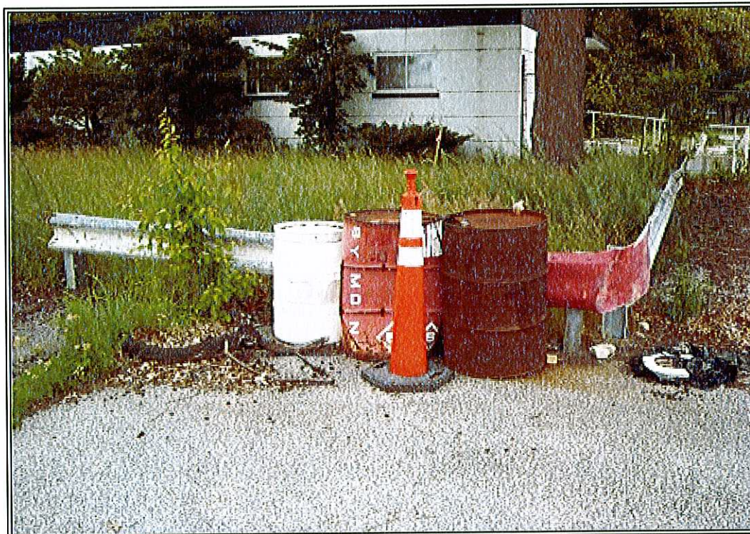
PHOTO 18: Three drums stored on-Site. The drums did not have any evidence of leaking, although they were bulging and warped. The only drum with a discernible label was the faded red drum, which was labeled "diesel fuel solution".
