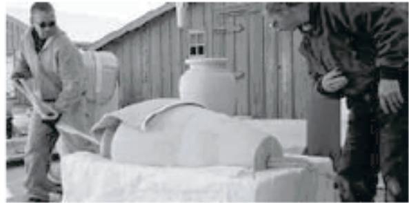
Attach both ends of the endless roundsling to equipment used for elevating. Pad the edges of the Urn with the supplied harness pads where the endless roundsling will come in contact with the Urn. See photographs.
