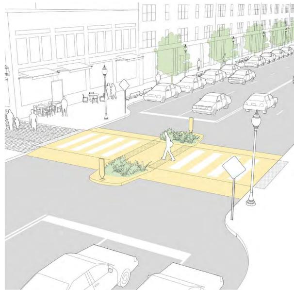
Tabletop intersections raise the entire intersection or crossing area to provide barrier free access (no ramps required). Use of this type of intersection will provide traffic calming by reducing vehicular speed around the park.
