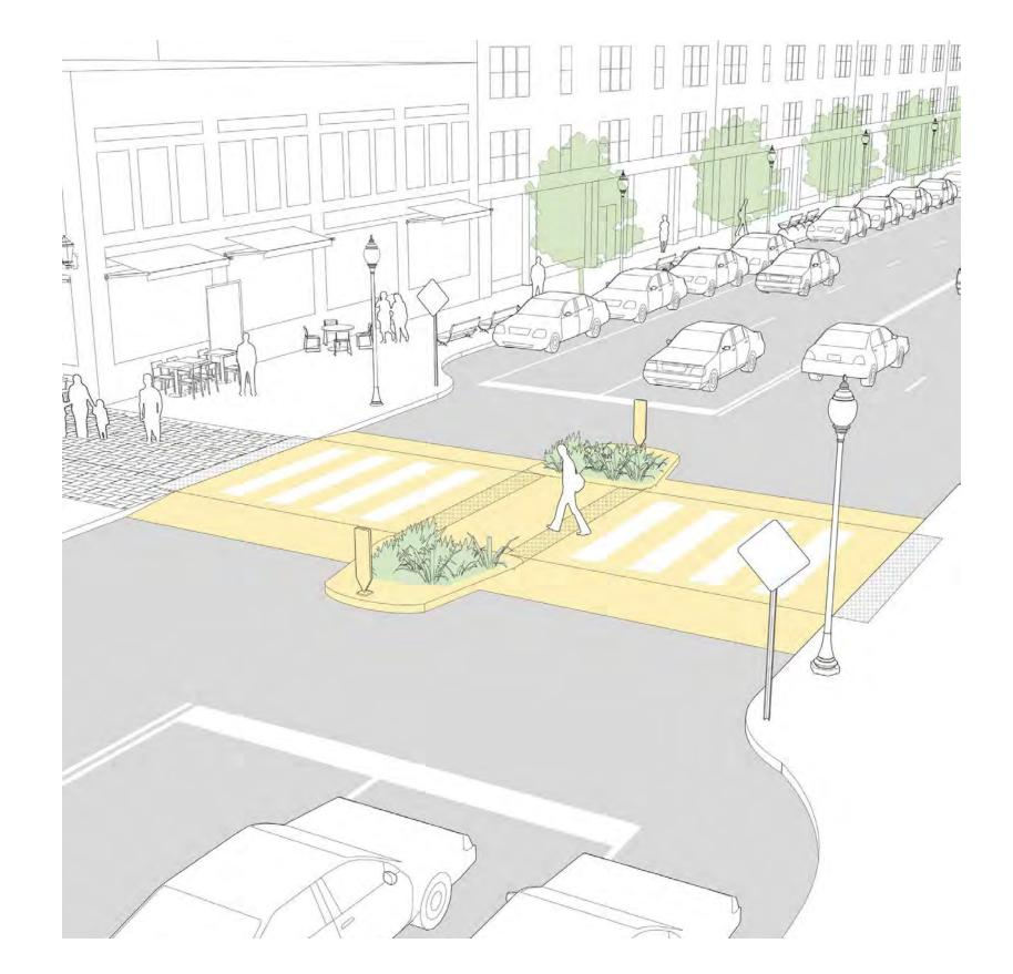
Tabletop intersections raise the entire intersection or crossing area to provide barrier free access (no ramps required). Use of this type if intersection will provide traffic calming by reducing vehicular speed around the park.
