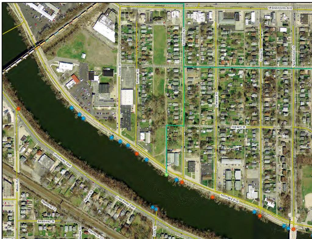
The yellow lines indicate combined sewer pipes. In general, flow travels from north to south. Once flow reaches Northside Boulevard, it flows through a 36" diameter pipe (yellow line that runs parallel to the river) and continues northwest. If flow exceeds the capacity of the 36" diameter pipe, the combined system will discharge into the St. Joseph River through CSO 33 (indicated by the red icon near Emerson Avenue) and CSO 35 (indicated by red icon near Clover Street).
