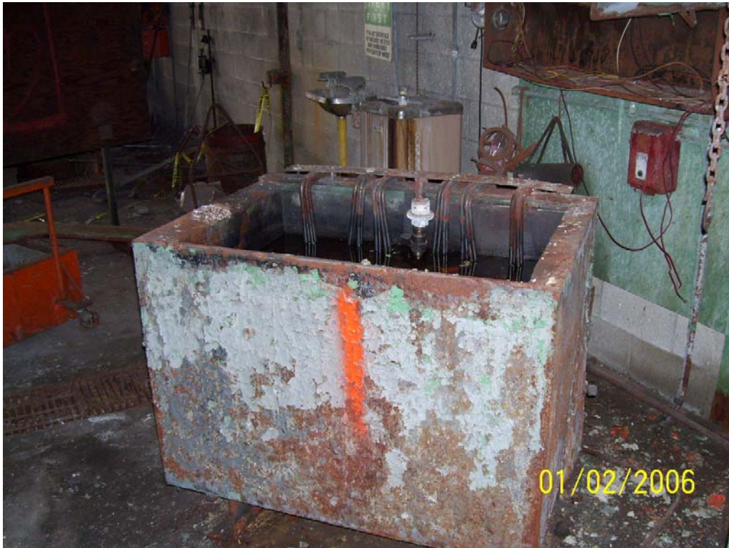
Site: South Bend Lathe Removal Photo Number: 5 Direction: Southwest Subject: Vat of caustic liquid, pH 11
